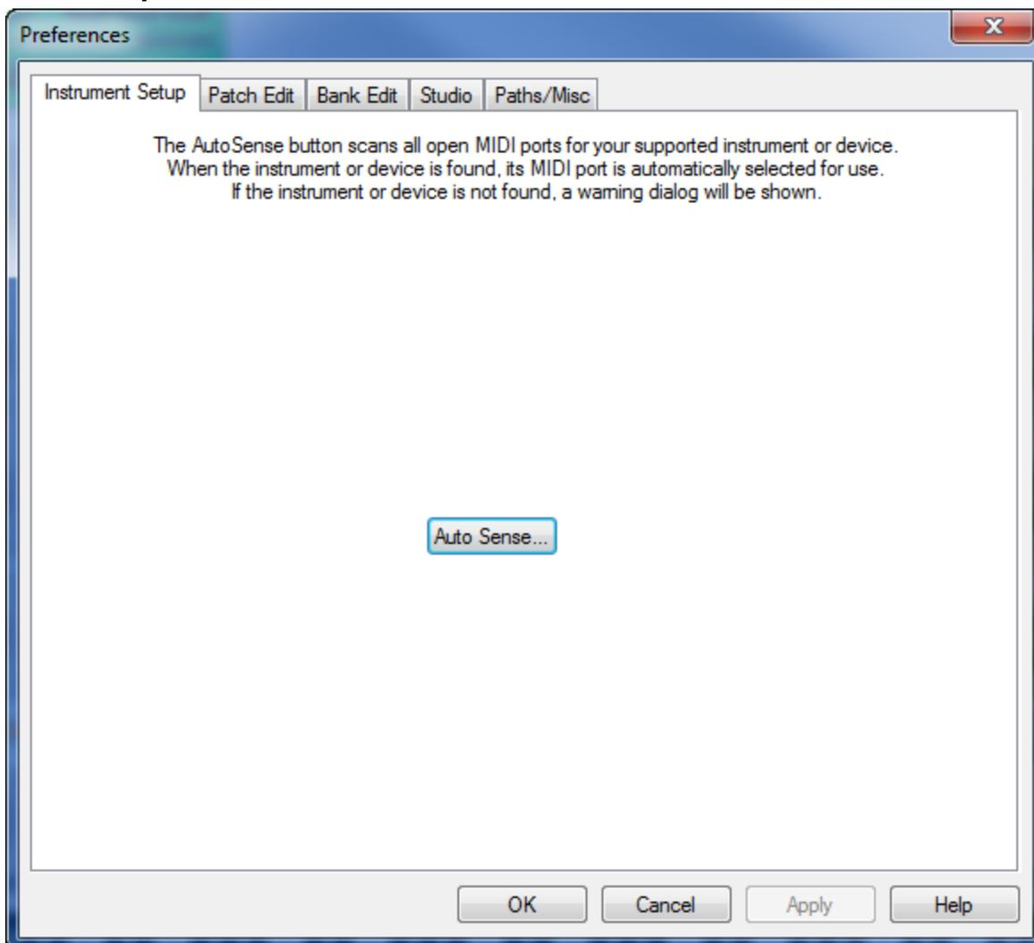
The first tab in the Preferences dialog is **Instrument Setup**: This tab contains the 'AutoSense' button that triggers the program to scan for Venom's existence on all MIDI ports selected for use by the editor software.
